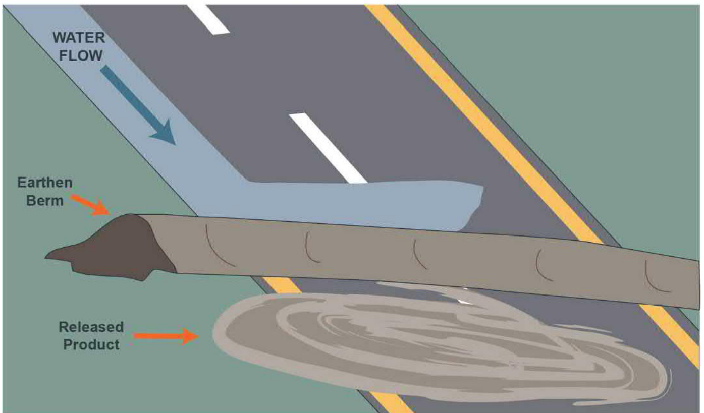
SURFACE FLOW DIVERSION
